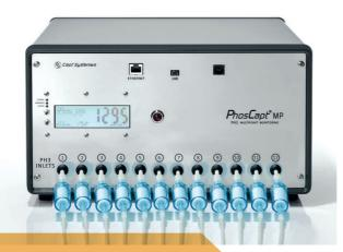
Dual gas sensor with automatic switching between high and low concentration sensors to monitor fumigation efficacy, degassing and security on 12 sampling lines up to 650 feet (200 m) in length.
